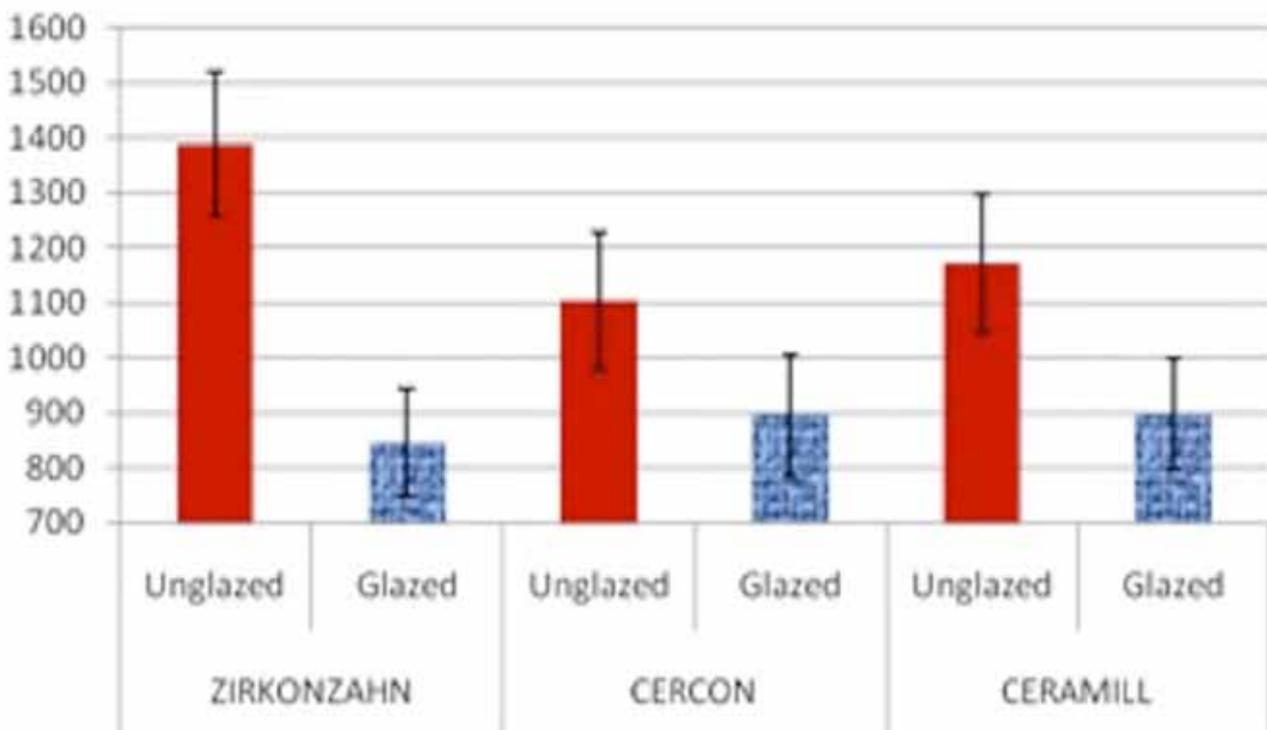
**Figure 1** - The mean biaxial flexural strength values (MPa) for zirconia systems with and without glazing.
