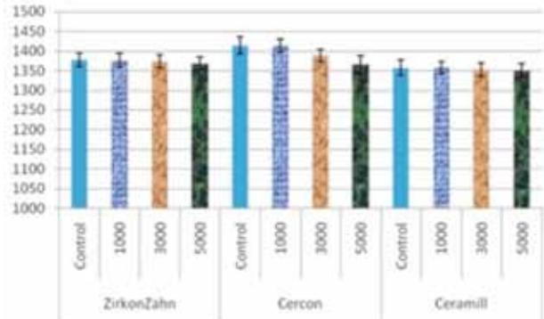
**Figure 4** - The mean Vickers hardness values (VHN) for unglazed glazed zirconia systems without and with thermal cycling.
