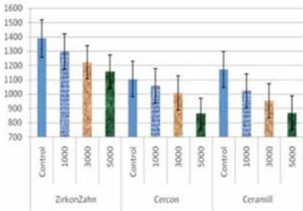
**Figure 2** - The mean biaxial flexural strength values (MPa) for unglazed zirconia systems without and with thermal cycling.
