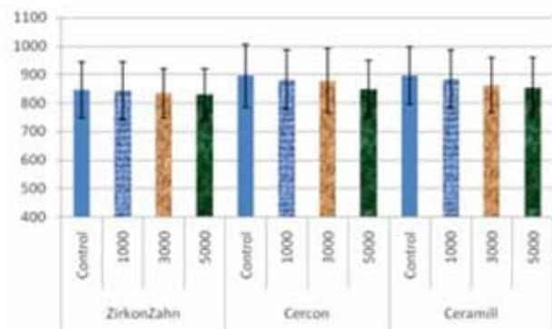
**Figure 3** - The mean biaxial flexural strength values (MPa) for glazed zirconia systems without and with thermal cycling.
