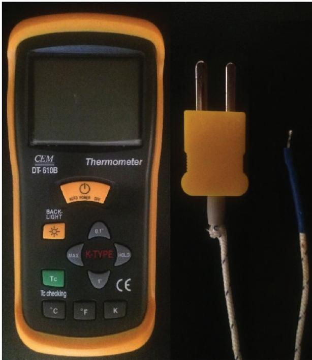
Figure 1 - Digital thermometer with double entrance thermocouple Model CEM DT-610B).
