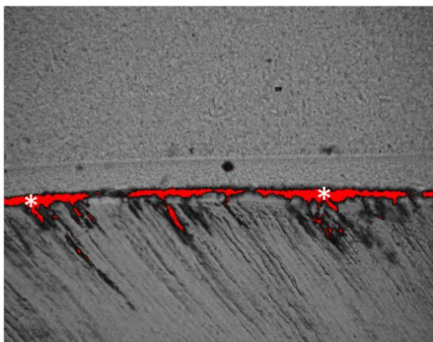
**Figure 1** - Image analysis for the area infiltrated by silver nitrate. \*The region of the interface is selected and the program interprets the points in red as infiltration area.
