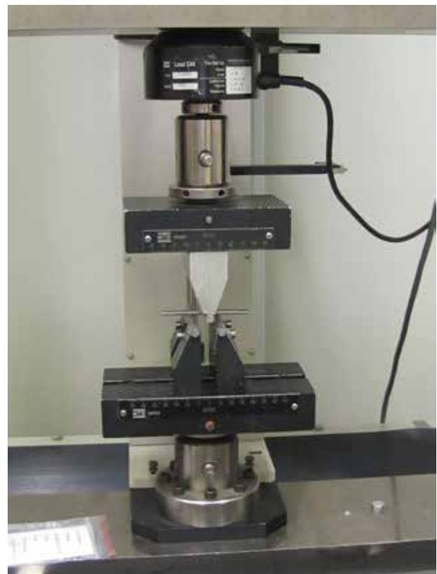
Figure 6 - Flexural strength test carried out by means of a universal testing machine set at 0.5 mm/min.
