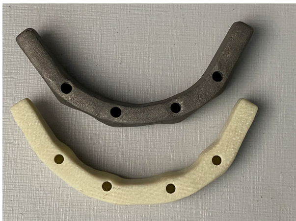
Figure 2 - Top view of Cobalt-chromium and Fiberglass bars in the finalization process.
