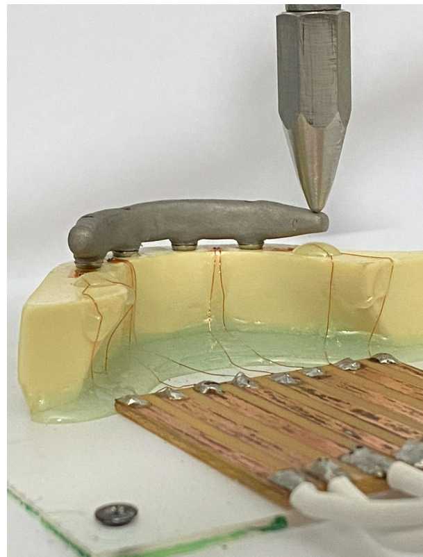
Figure 4 - Test specimen finished with Cobalt-Chromium bar subjected to static compression with a force of 100N on the right cantilever end.
