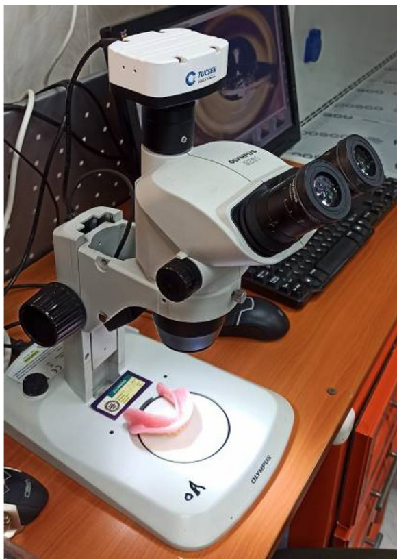
Figure 4. The stereomicroscope (Olympus SZ61, Japan) beside the camera (10MP Tucsen USB2.0 H series, ISH 1000, China).
