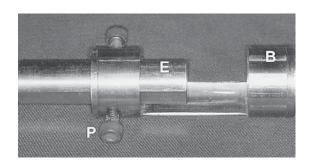
**FIGURE 2** – Gadget developed to blocking the coping on the master die: (P) fixing screw; (E) piston; (B) base.
