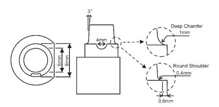
FIGURE 1 - Schematic drawing of the master dies.
