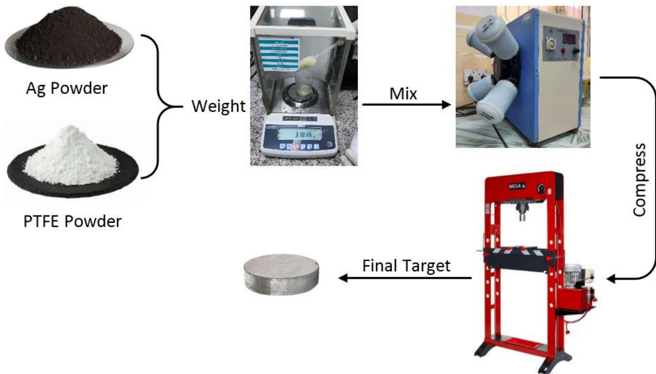
Figure 1 - Preparation steps of RF target.
